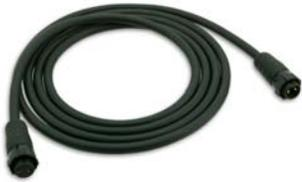
SPEN cords are designed for use with Meyer Sound's MM-4 speakers and utilize 2-pole EN3 water-resistant connectors. Manufactured in a variety of standard lengths, SPEN cords are available in both link and extension cable configurations. Each assembly features two 16-gauge, 26-strand conductors in a round, matte-finish flexible jacket to deliver high-quality speaker level signals with minimal signal loss.
