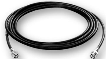
BC Series cords are coaxial cable assemblies with a BNC connector on each end. Two cable types are available: RG58/U (50 ohms) used for RF signals, and RG59/U (75 ohms) for video use. The BNC connectors are crimp-type to assure accurate and reliable connections.
